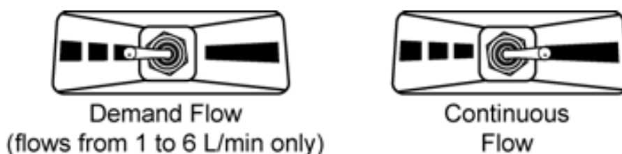
Figure 17: Continuous/Demand Flow Switch
